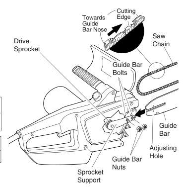
Figure 3 - Assembling Guide Bar, Chain, and Hand Guard
